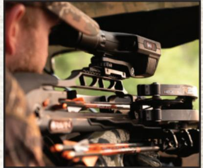
Loosen the Torx head bolts on the base of the mount using the provided T25 Torx® wrench until the clamping bars open enough to straddle the rail. Position the Oracle X mount on the rail of your crossbow so the crossbow and the Oracle X are in a comfortable shooting position for your eye.
