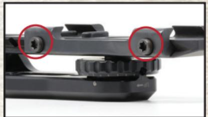
With the clamping nuts loose, push the scope forward until there is firm metal to metal contact on the recoil lug. Tighten both bolts to 40 to 70 in-lbs.
